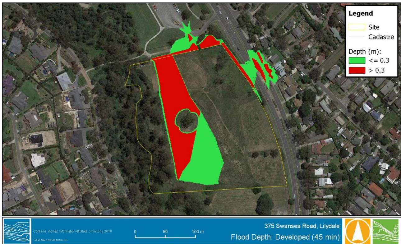
Figure 3-9 Developed Conditions 1% AEP Peak Flood Depths - from Local External Catchment
