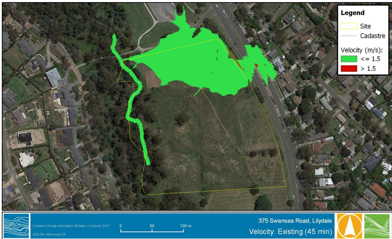
Figure 3-10 Existing Conditions 1% AEP Peak Flood Velocity - from Local External Catchment
