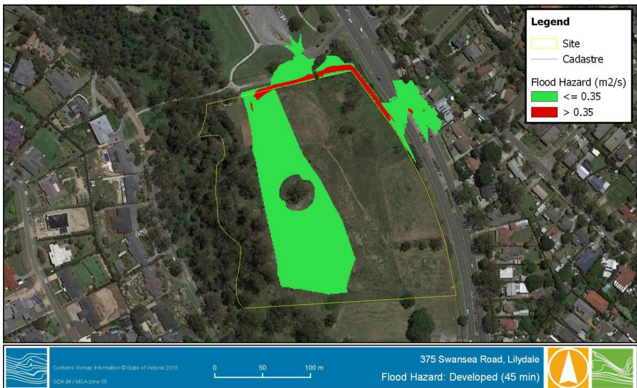
Figure 3-13 Developed Conditions 1% AEP Peak Flood Hazard (Depth x Vel) - from Local External Catchment
