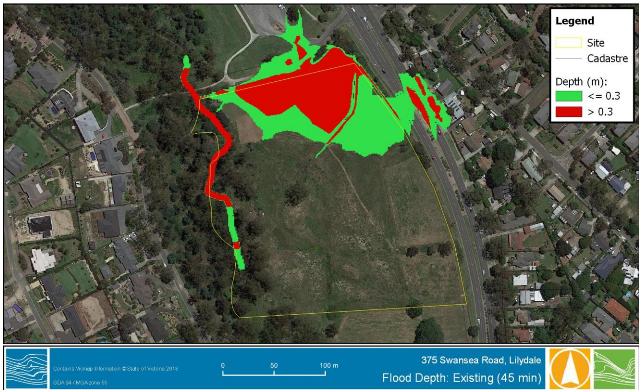
Figure 3-8 Existing Conditions 1% AEP Peak Flood Depths - from Local External Catchment
