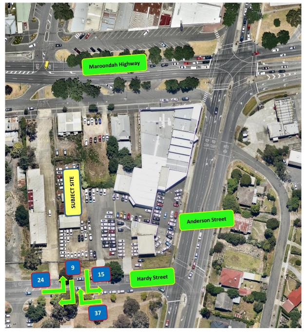
Figure 25: AM Peak Hour – Forecast Traffic Movements at Hardy Street Access Point (vehicles per hour)
