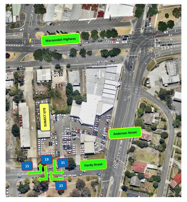
Figure 26: PM Peak Hour – Forecast Traffic Movements at Hardy Street Access Point (vehicles per hour)
