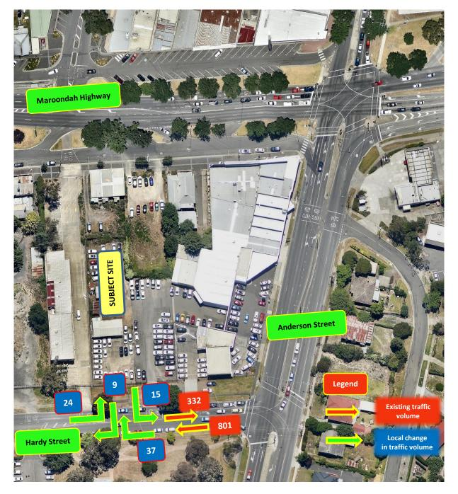
Figure 27: AM Peak Hour - Comparison of Development Traffic & Existing Traffic at Hardy Street Access Point
