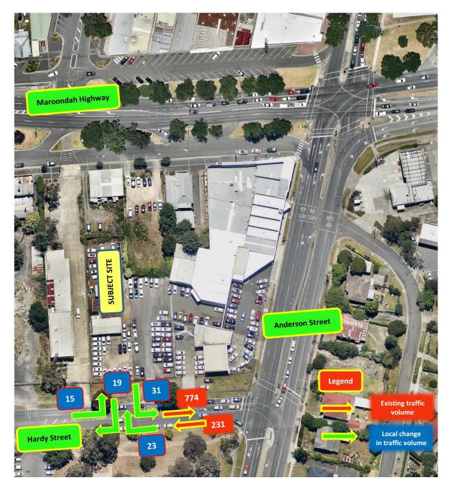
Figure 28: PM Peak Hour – Comparison of Development Traffic & Existing Traffic at Hardy Street Access Point
