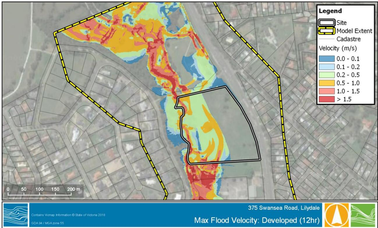
**Figure 4-7 Flood Velocities under the Development Scenario**
