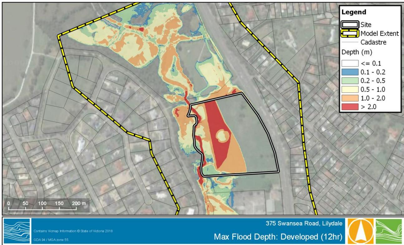
**Figure 4-6 Flood Depths under the Development Scenario**
