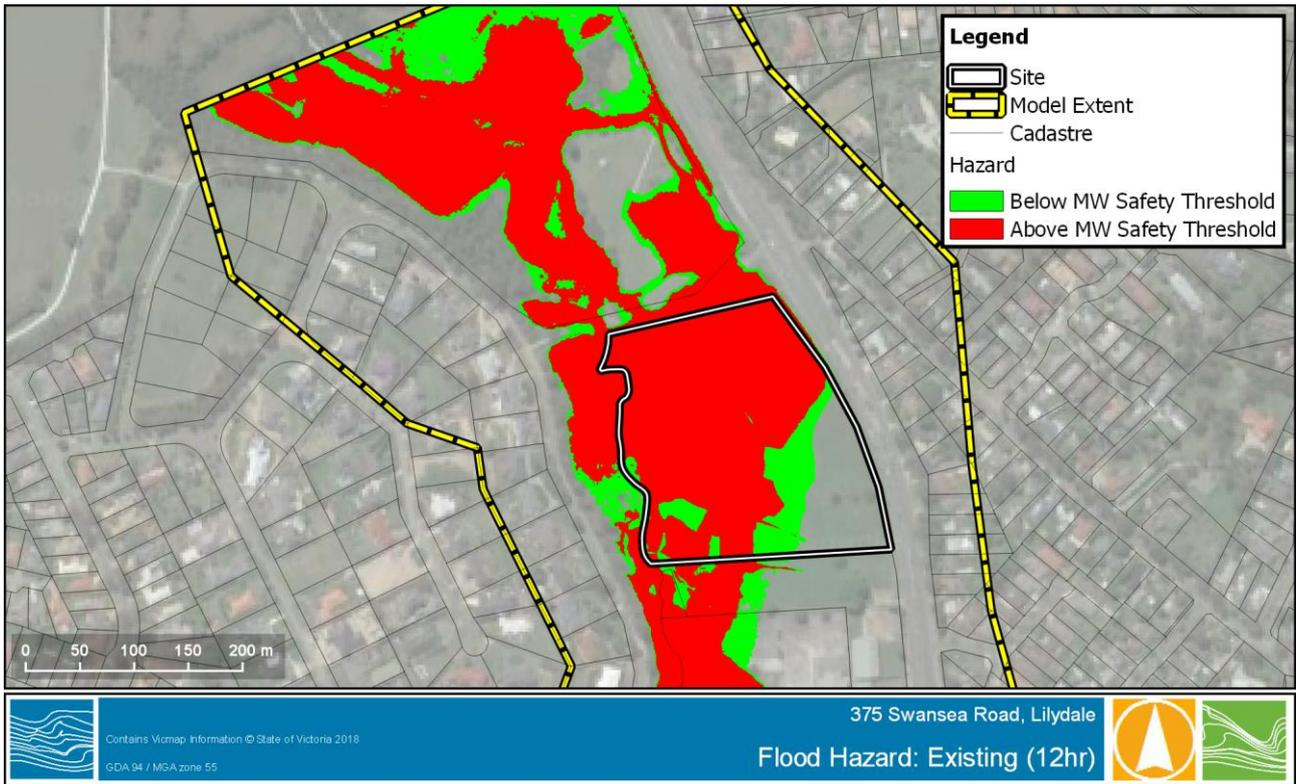
Figure 5-1 Flood Hazard under the Existing Scenario
