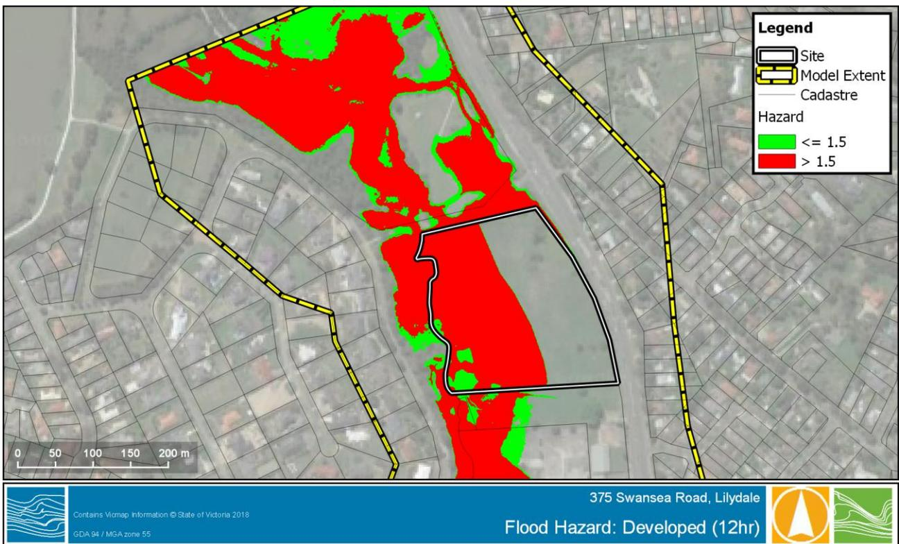
Figure 5-2 Flood Hazard under the Development Scenario
